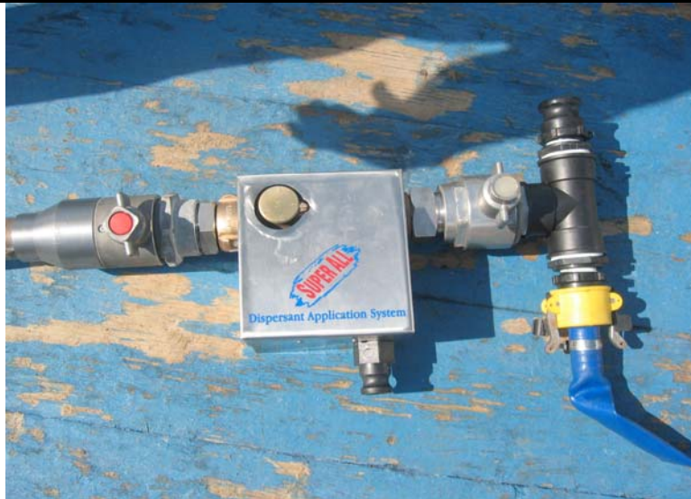
Fig. 1 . SuperAll Dispersant Application System(1%-6%)
